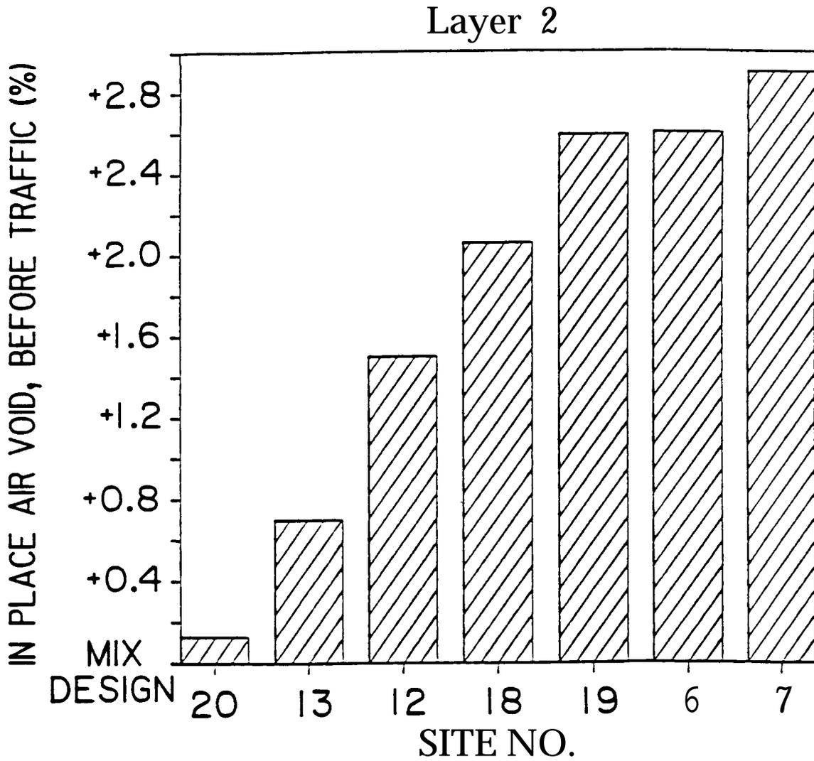
Figure 15. Comparison of Quality Control Air Void Contents Obtained Prior to Traffic to Their Mix' Design Air Void Contents for Layer 2 Mixtures
