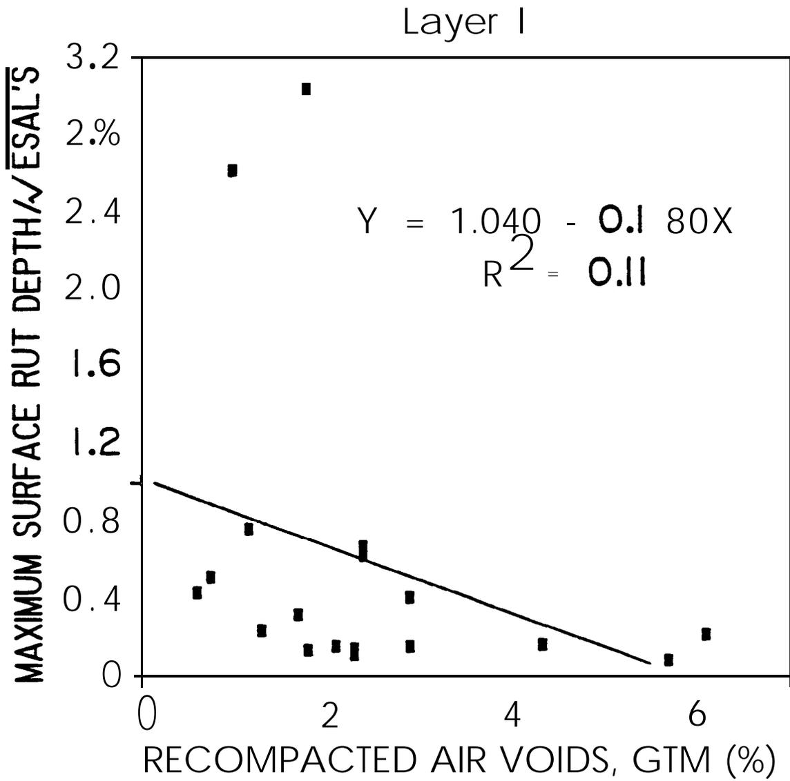
Figure 3. GTM Recompacted Air Void Content vs Maximum Surface Rut Depth  $\div$  Square Root of Traffic in Million ESAL's
