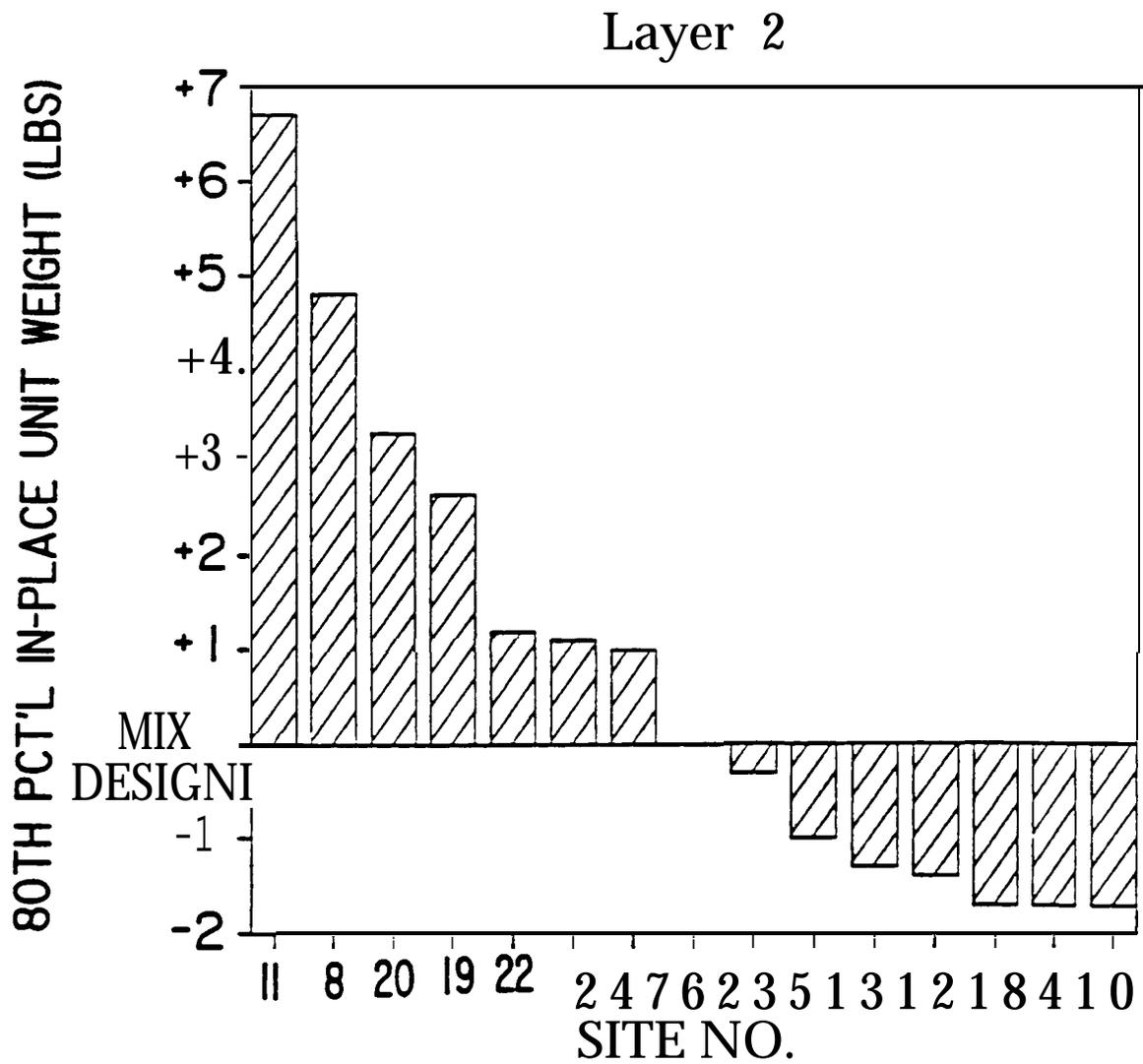
**Figure 13. Comparison of 80th Percentile In-Place Unit Weights to Their Mix Design Unit Weights for Layer 2 Mixtures**
