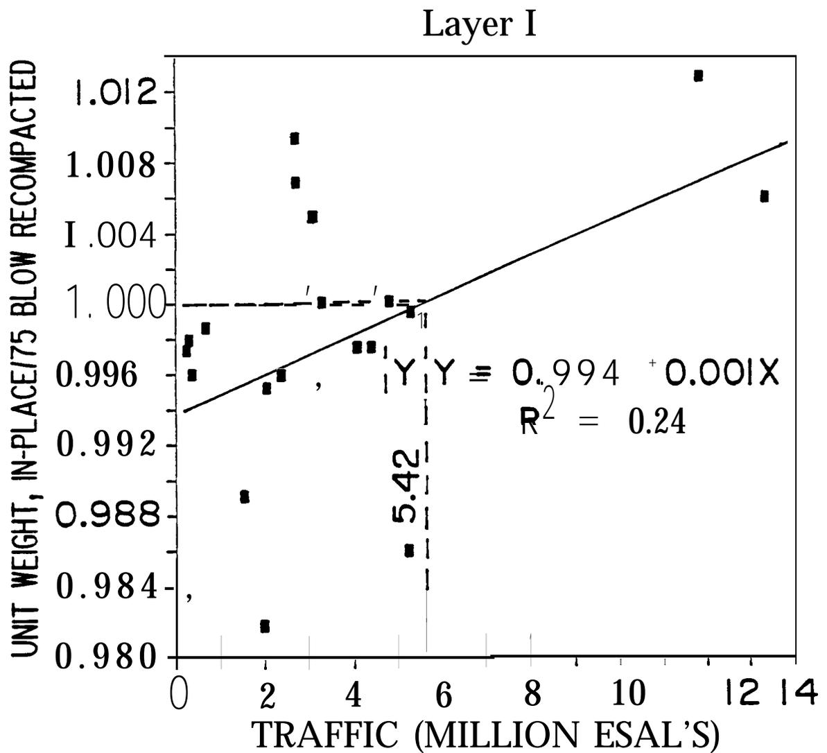
Figure 8. Traffic vs. Ratio of In-Place to 75 Blow Recompacted Unit Weight for Layer 1 Mixtures
