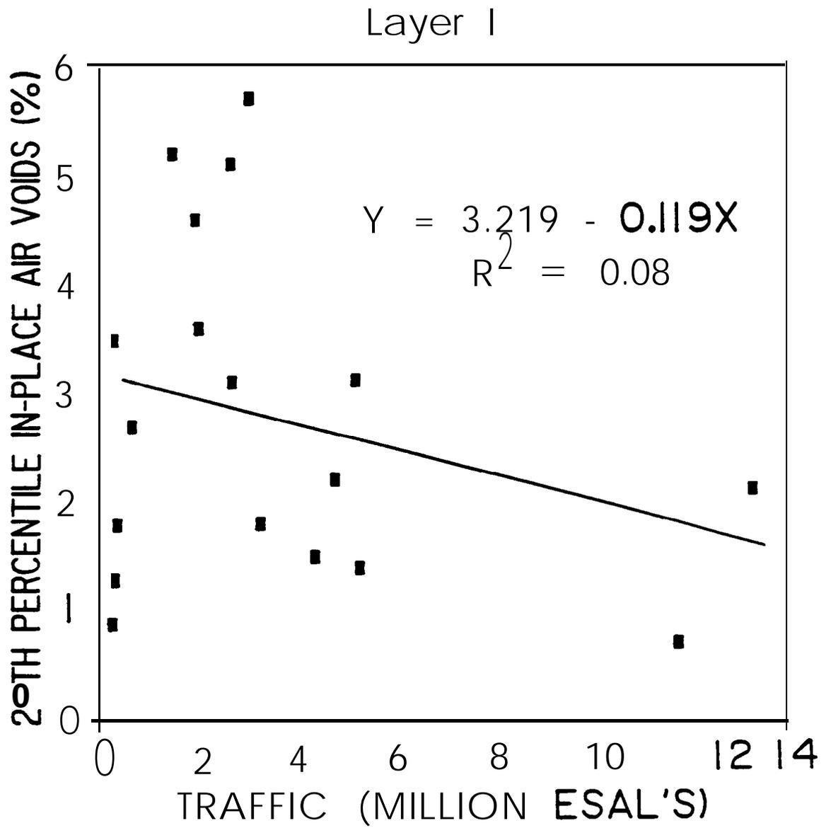
Figure 4. Traffic vs. 20th Percentile In-Place Air Void Content for Layer 1 Mixtures
