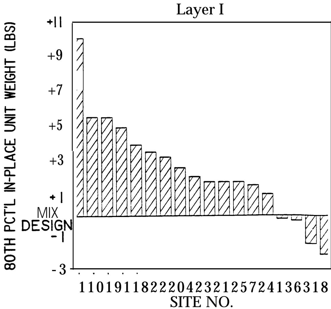
Figure 12. Comparison of 80th Percentile Unit Weights to Their Mix Design Unit Weights for Layer 1 Mixtures
