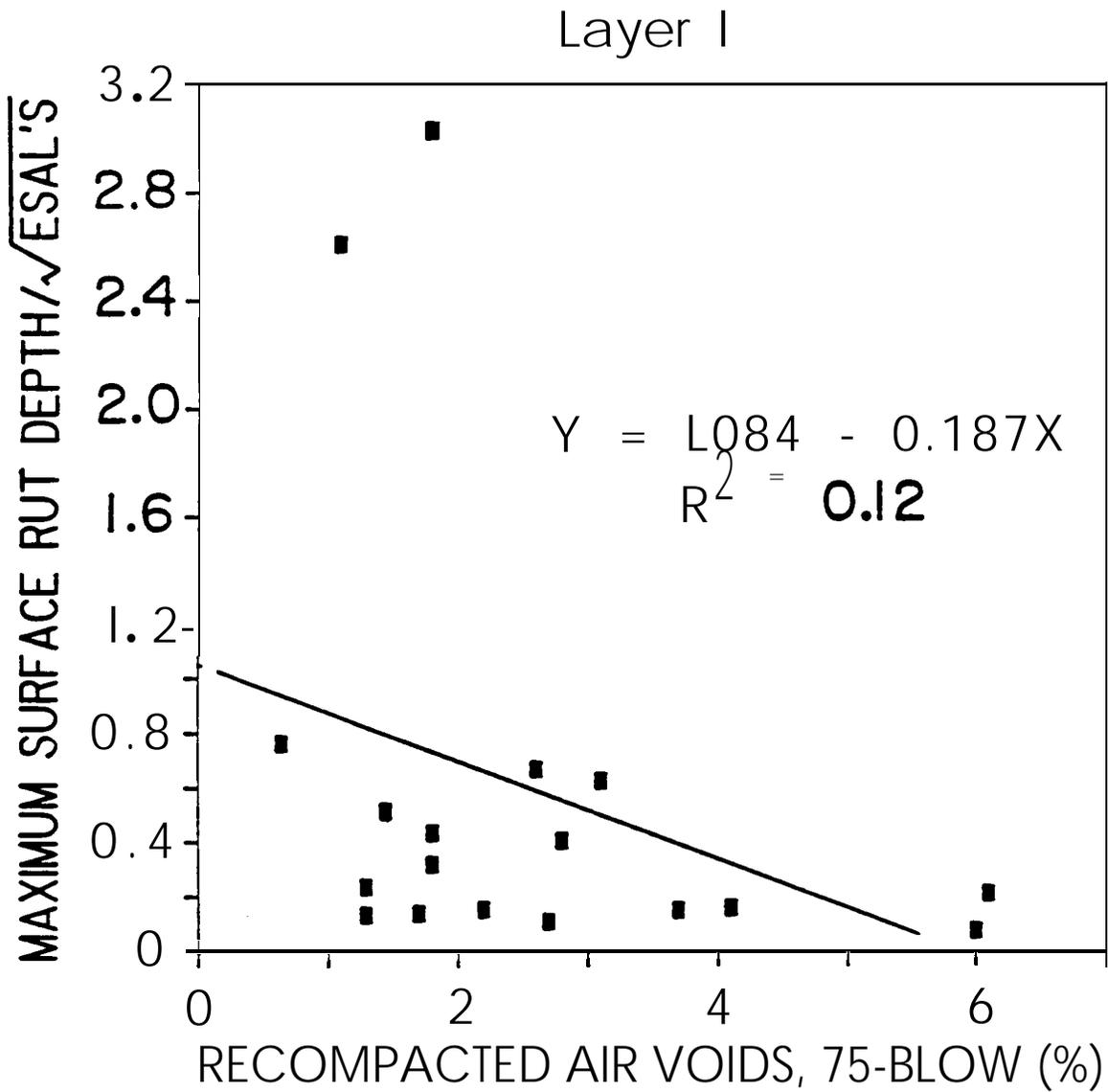
Figure 2. 75-Blow Recompacted Air Void Content vs Maximum Surface Rut Depth  $\div$  Square Root of Traffic in Million ESAL's
