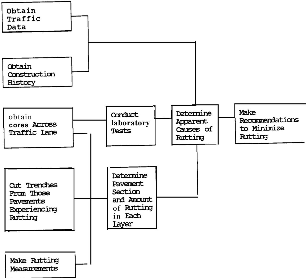
Figure 1. Overall Test Plan
