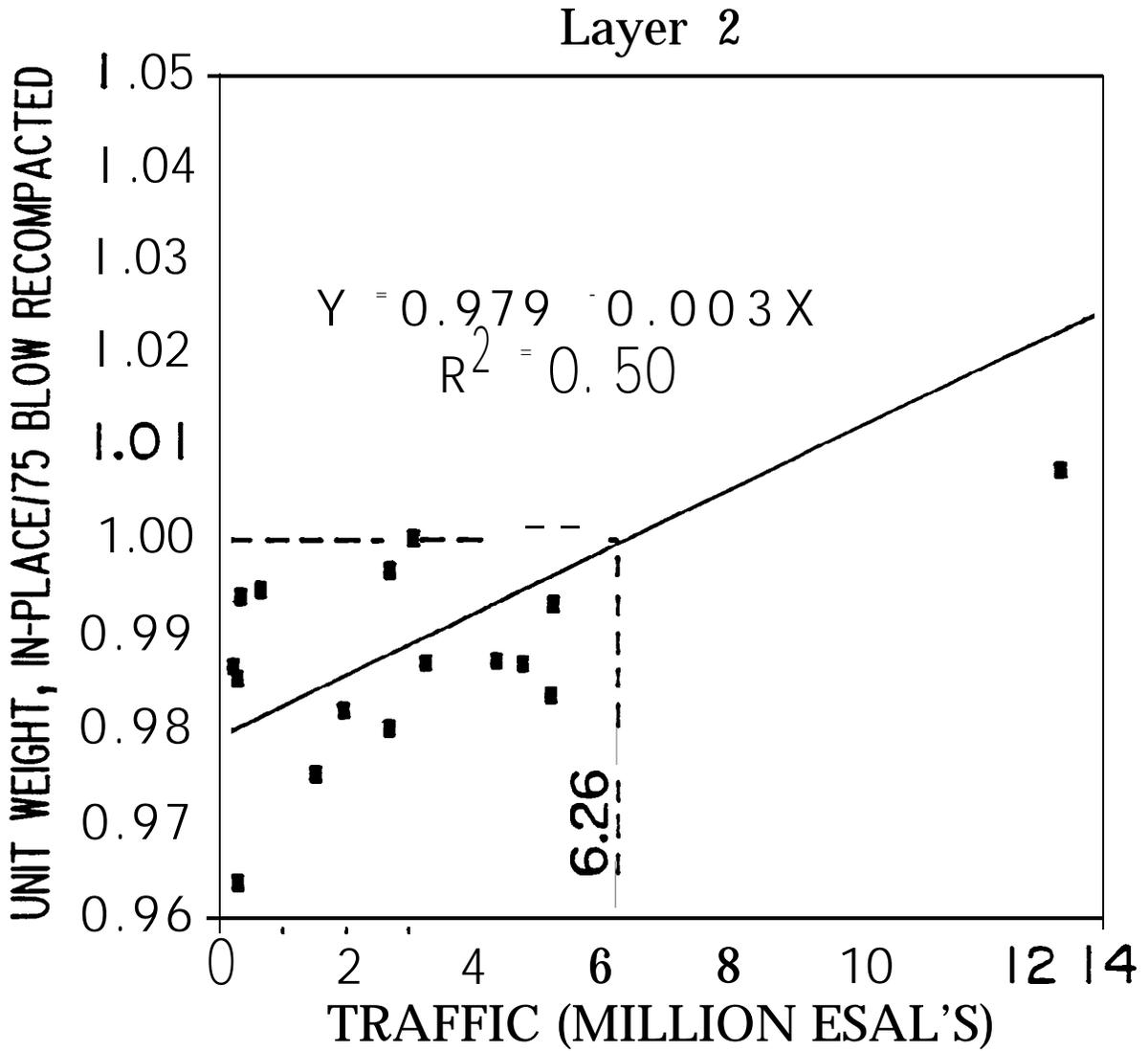
Figure 9. Traffic vs. Ratio of In-Place to 75 Blow Recompacted Unit Weight for Layer 2 Mixtures
