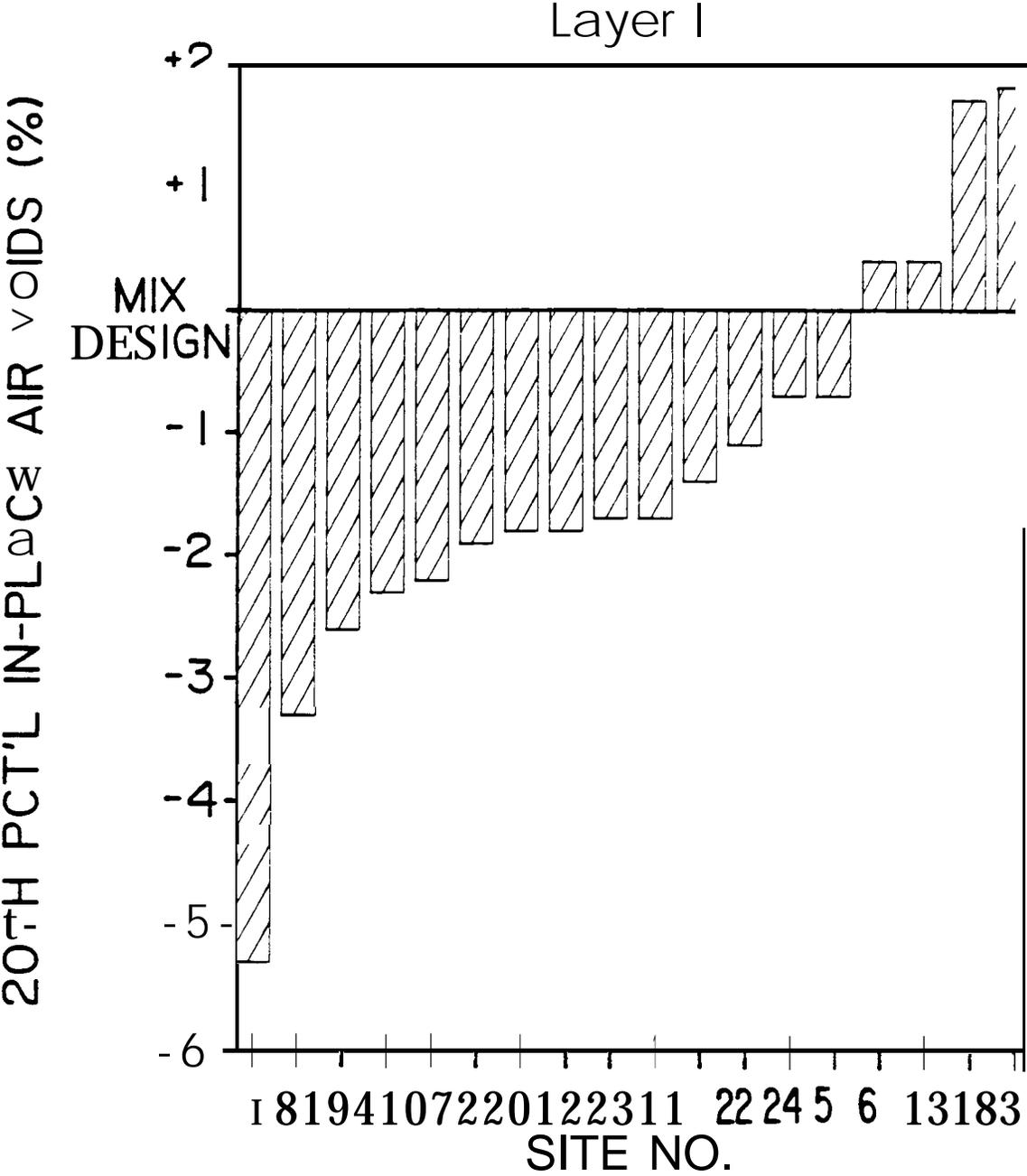
Figure 10. Comparison of 20th Percentile In-Place Air Void Contents to Their Mix Design Air Void Contents for Layer 1 Mixture
